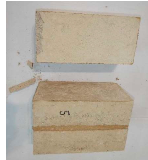
Shear failure at block-mortar interface
